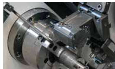
Chuck Air Blow (Upper Chuck)
