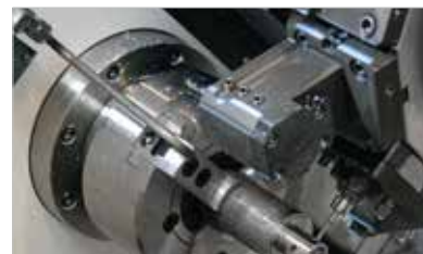
Chuck Air Blow (Upper Chuck)
