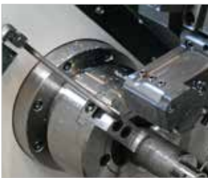
Chuck Air Blow (Upper Chuck)
