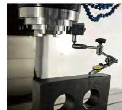
X / Y axis verticality : 0.010/500mm
