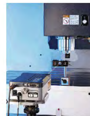
Laser measurement pitch: Standard measurement compensation.
