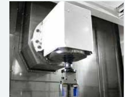
Tool spindle gripper type parts catcher
